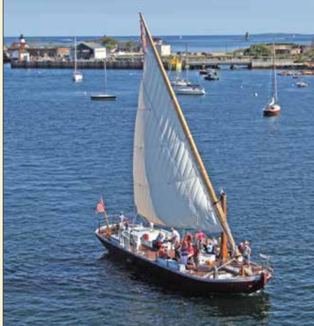
PISCATAQUA's single sail measures approximately 900 sq ft in area. East Boothbay, Maine, sailmaker Nathaniel S. Wilson built it of Oceanus sailcloth—a synthetic fabric whose look and feel are of canvas.
