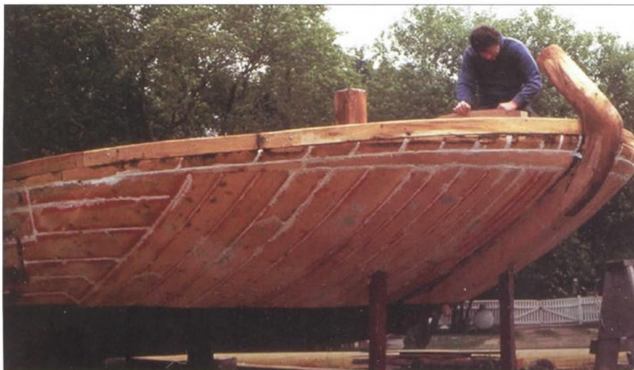
In keeping with tradition, most of this gundalow is fastened with 5,000 trunnels. Note the spoon bow.
